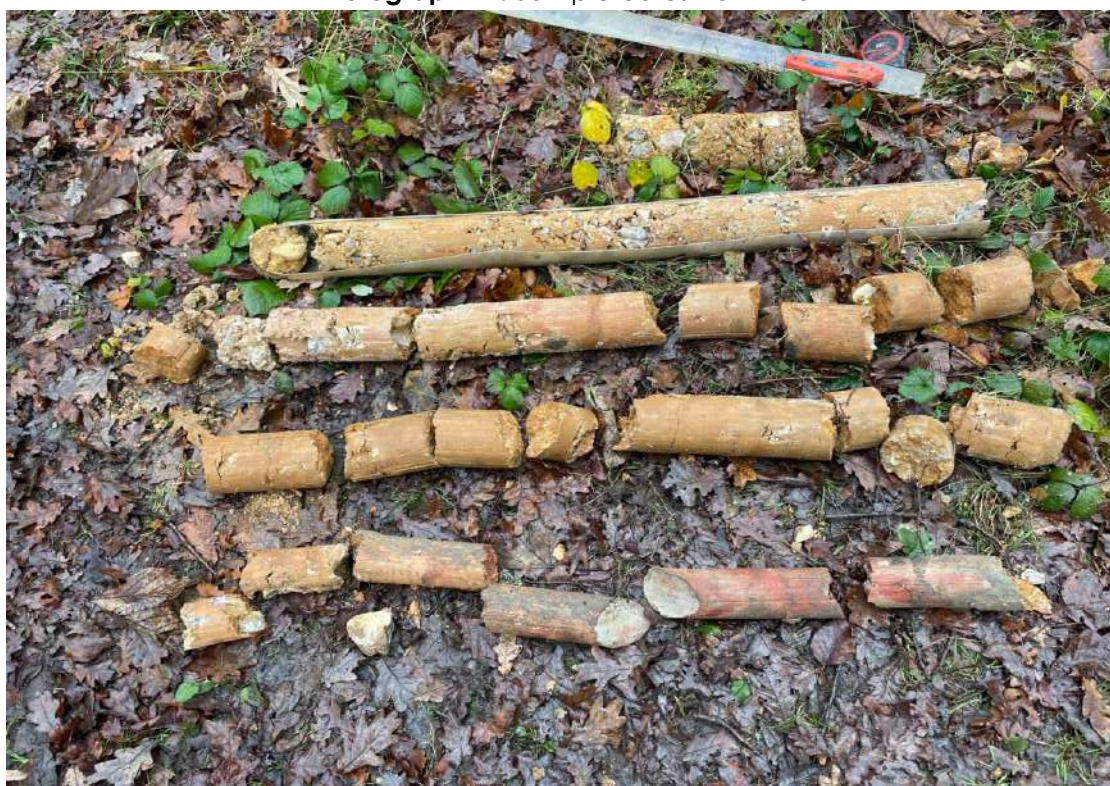
Photograph 12: Sample cores from BH6
